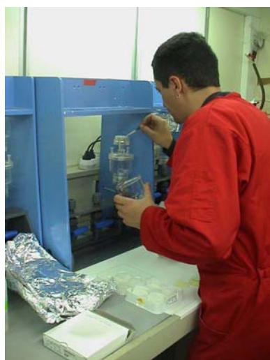
System for size fractionated particulate phosphate measurements
