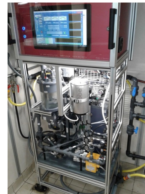
Ferry-box (wave, currents, salinity, temperature, viscosity)
