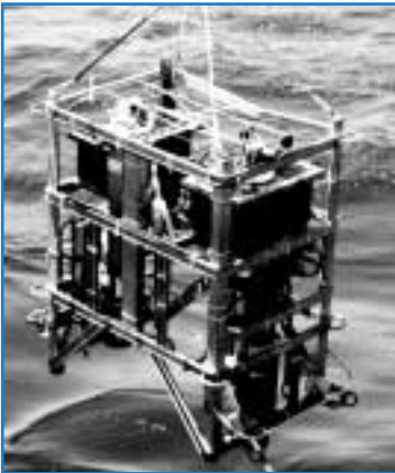
Figure 1. The Underwater Video Profiler (UVP) instrument package presented here includes the underwater imaging system, an SBE CTD, a fluorometer and nephelometer both from Chelsea Instruments.
