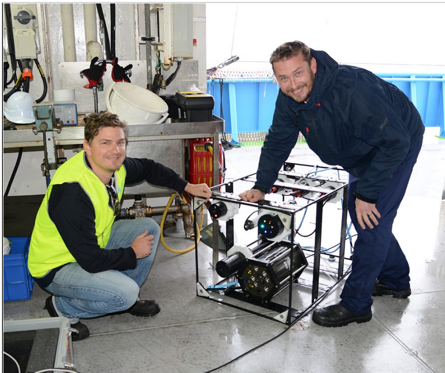
Dr Matthew Slivkoff (In situ Marine Optics) and Dr Wojciech Klonowski (In situ Marine Optics) indicating the components of their IOP (Inherent Optical Properties) package which they have just retrieved after collecting measurements in the south-east Indian Ocean. Photo: Micheline Jenner AM.
