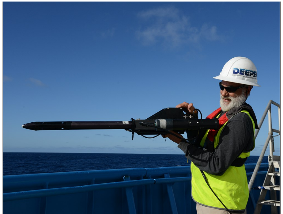
Charles Kovach (NOAA, USA) prepares to deploy a HyperPRO in-water profiling radiometer for establishing the underwater light profile in the tropical south-east Indian Ocean. Photo: Micheline Jenner AM.
