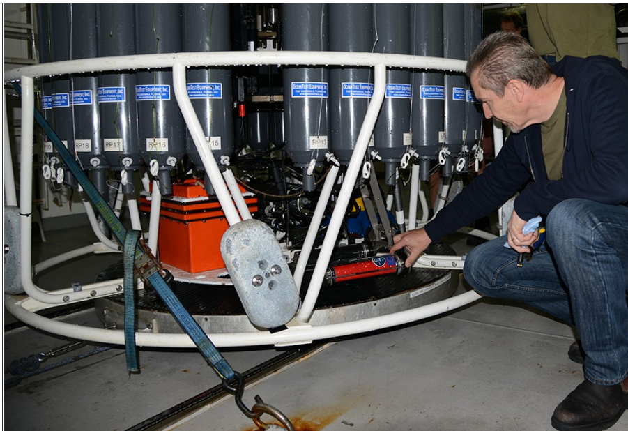
In the CTD room, Prof David Antoine (Curtin University) checks the UVP (two red cylinders) at the base of the CTD. Photo: Micheline Jenner AM.
