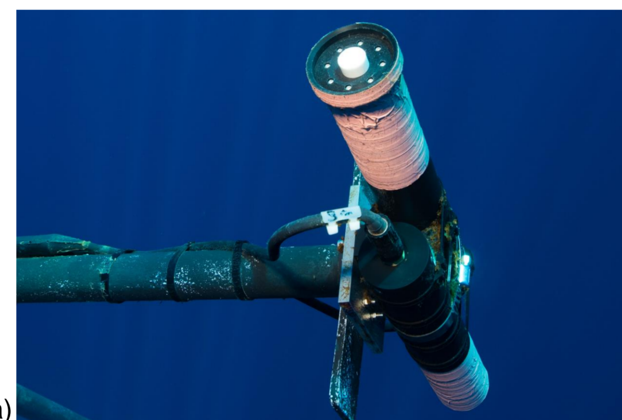
Fig.1: a) Hyperspectral radiometers on the buoy measuring Ed and Lu at 9m depth. b) Examples of data from hyperspectral radiometers at 4m and 9m: median Ed-spectra of 1 minute record.
