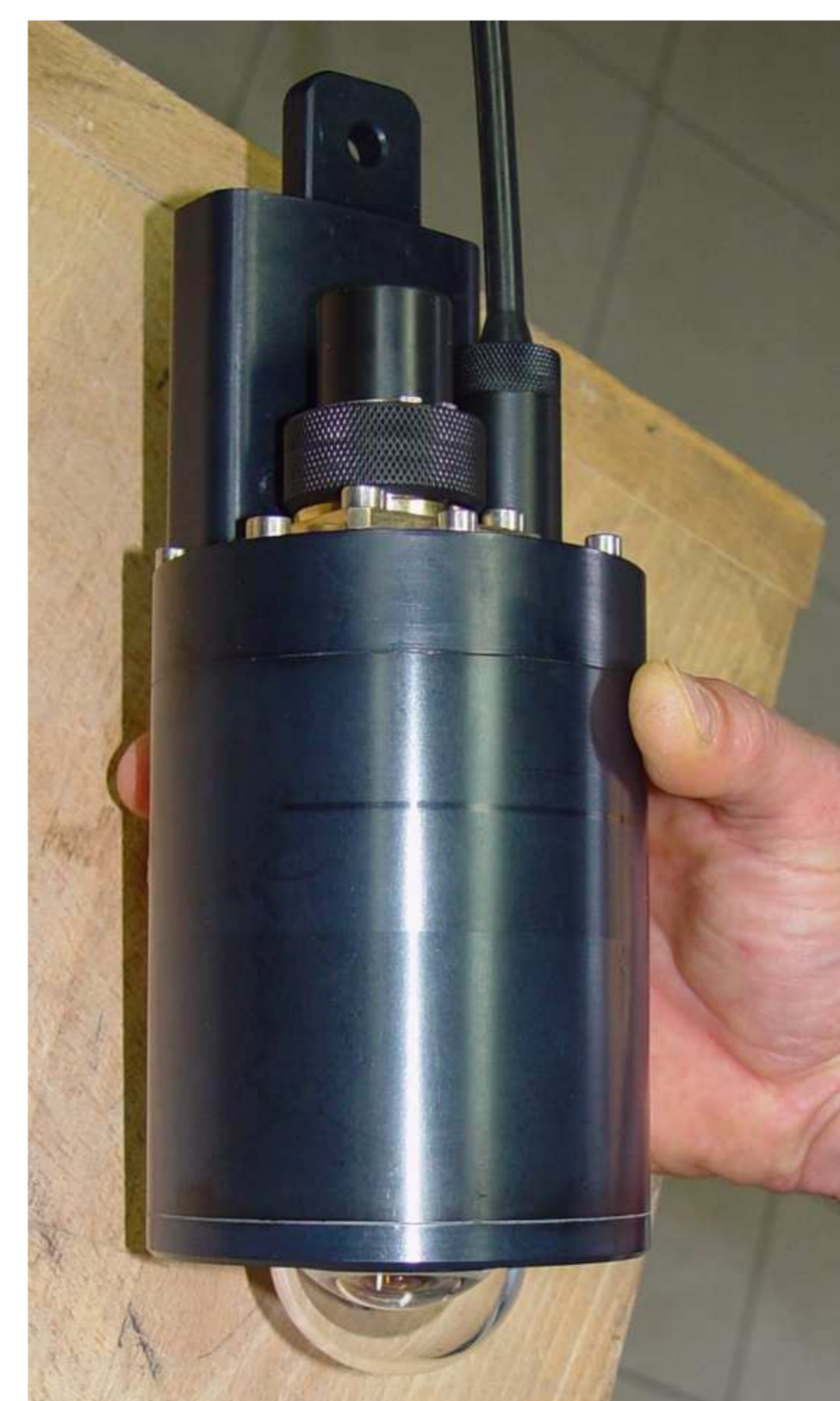
The radiance Camera
