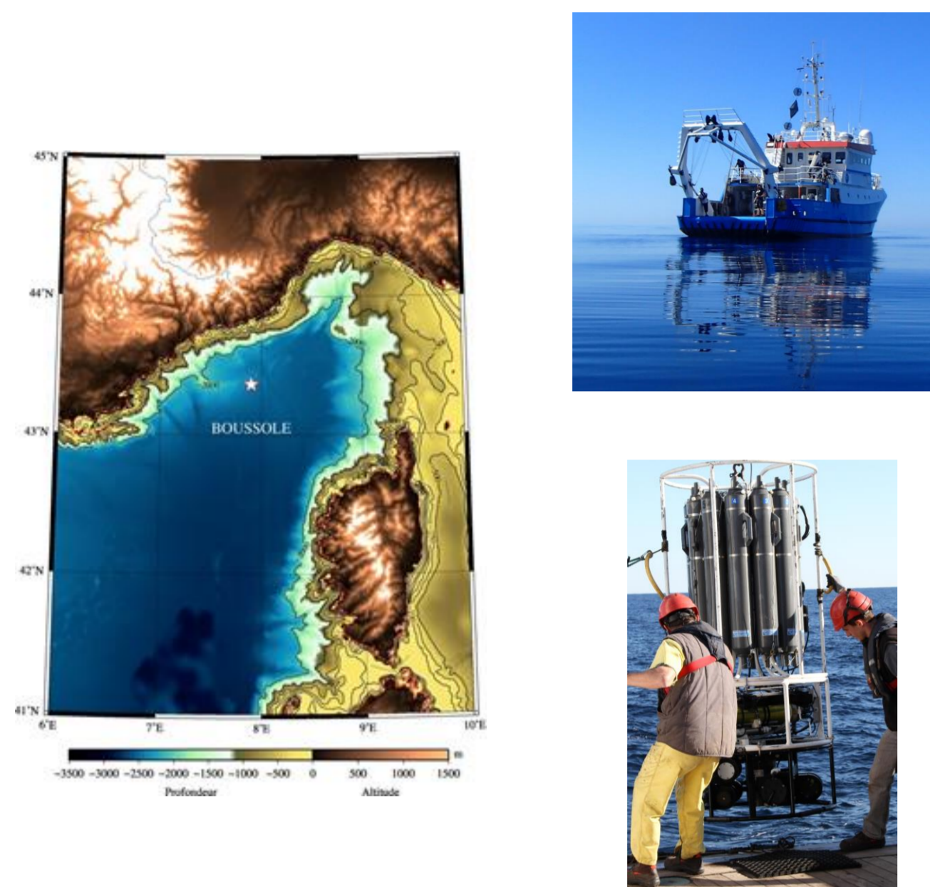
Fig.1 : Map of the NW Mediterranean Sea showing the location of the BOUSSOLE site (left). R/V Tethys II and CTD Rosette + IOPs package deployment at the BOUSSOLE site (right).
