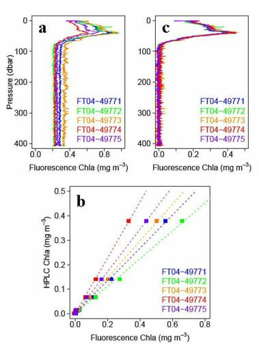
**Fig. 1.** The cross-calibration procedures of tag fluorometers at BOUSSOLE site (Western Mediterranean Sea, 7.9°E, 43.37°N). Fig. 1a shows the raw (uncalibrated) fluorescence profiles of five tags. Fig. 1b shows the linear regression analysis between fluorescence and HPLC Chl *a* concentration. Fig. 1c shows the calibrated fluorescence profiles.
