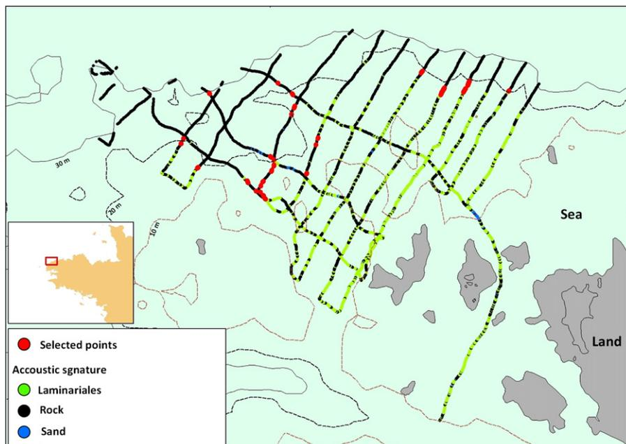
**Fig. 12.** Single-beam survey lines (thick lines) for the site Abers. Green dots denote the presence of kelp forest. Red dots are deepest occurrences of kelp forest.
