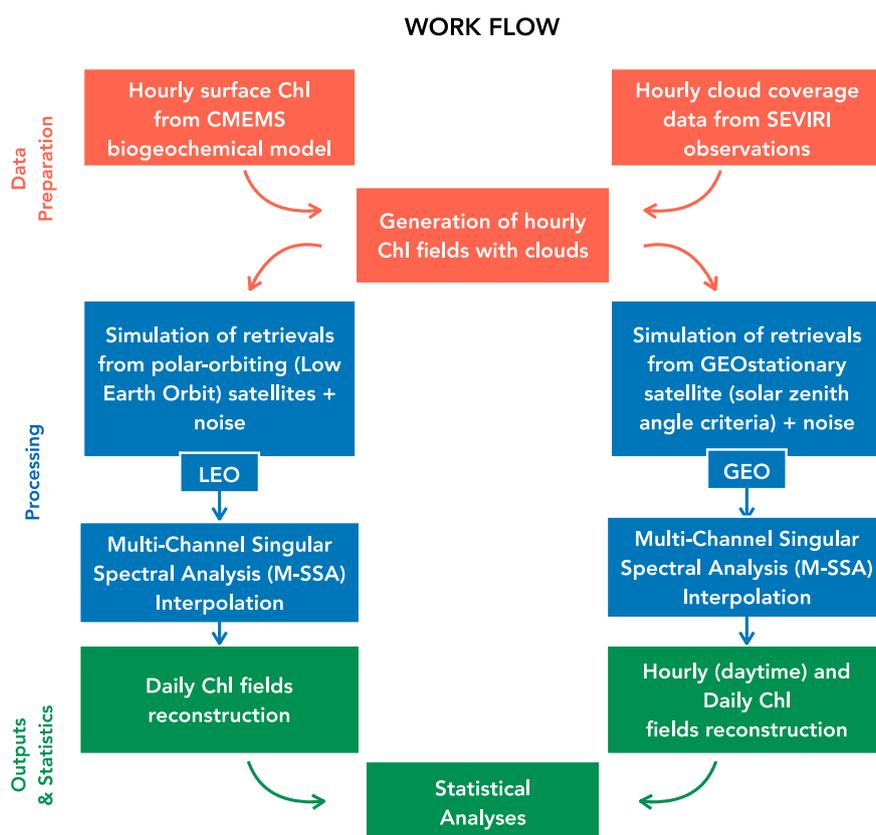
**Figure 1.** Flowchart diagram of the method developed in this paper. Orange represents dataset preparation, blue represents the processing of data, and green represents the outputs and statistical analyses.
