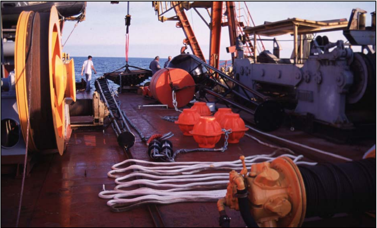
Fig. 7. The complete mooring line on the deck of the Castor-02 , before deployment. The beginning of operations started 20 July 2000, 0700 Greenwich Mean Time (GMT).
