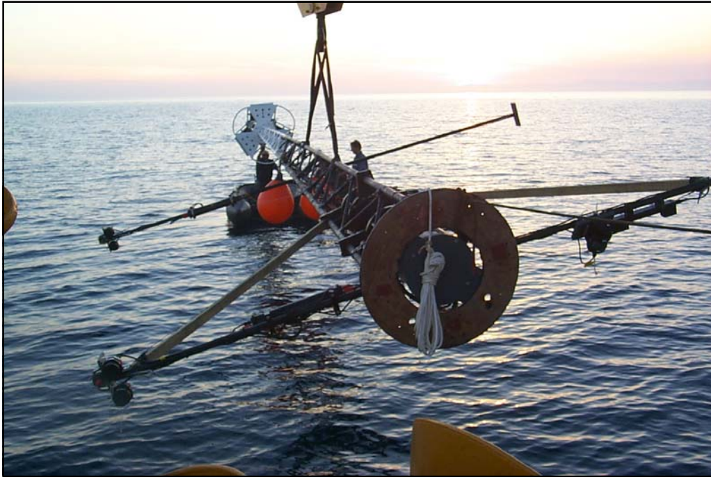
Fig. 10a. The upper superstructure of the buoy (Fig. 6) prior to it being fastened to the lower superstructure, which is done under water by divers. The optical sensors are visible at the end of the sensor arms in the left half of the picture. The two oblique arms are only used during deployment, to secure the buoy arms; they are removed after the buoy is deployed.
