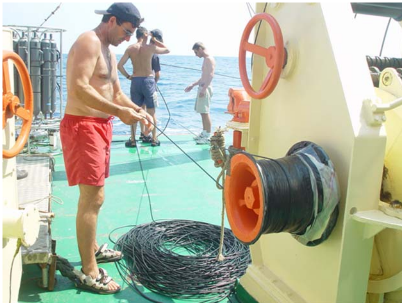
Fig 1. Hauling in the SPMR on the capstan.
