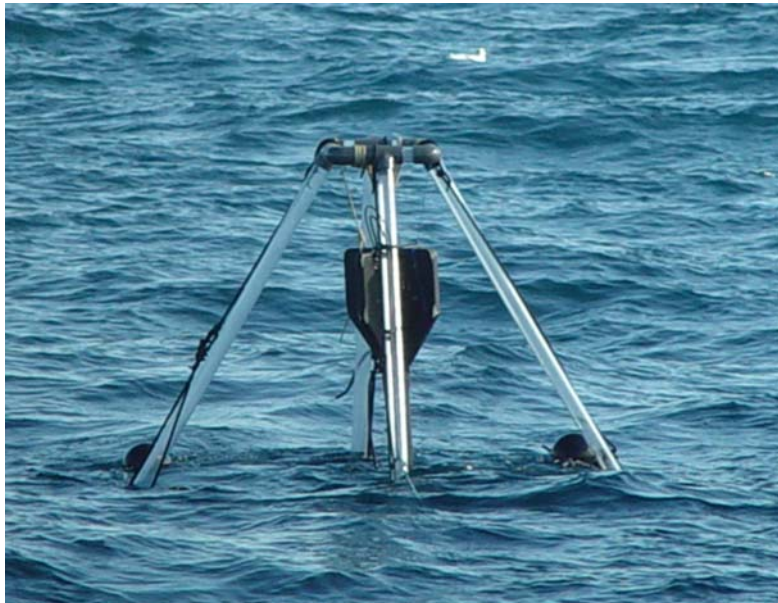
Fig 1. SPMR surface float apparatus for acquiring Eu data at approximately 20cm below surface. Data can be used to support near-surface extrapolation algorithms.
