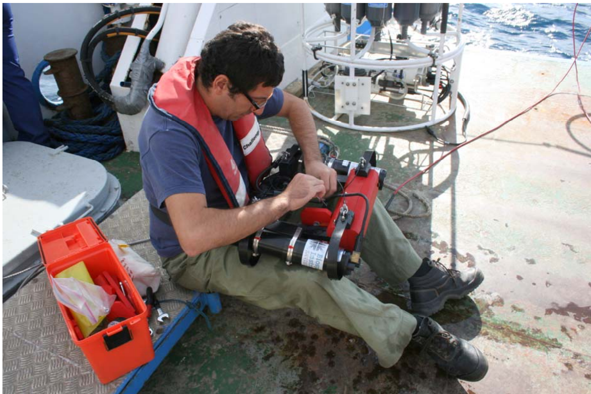
Figure 1. Vincenzo Vellucci making adjustments on the Biospherical C-OPS for a better balance of the instrument during the descent phase.
