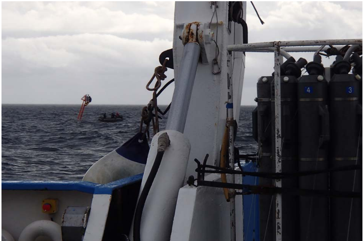
The CTD Rosette on the R/V Téthys II deck and V.Vellucci on the top of the BOUSSOLE buoy for data retrieval, on the background.
