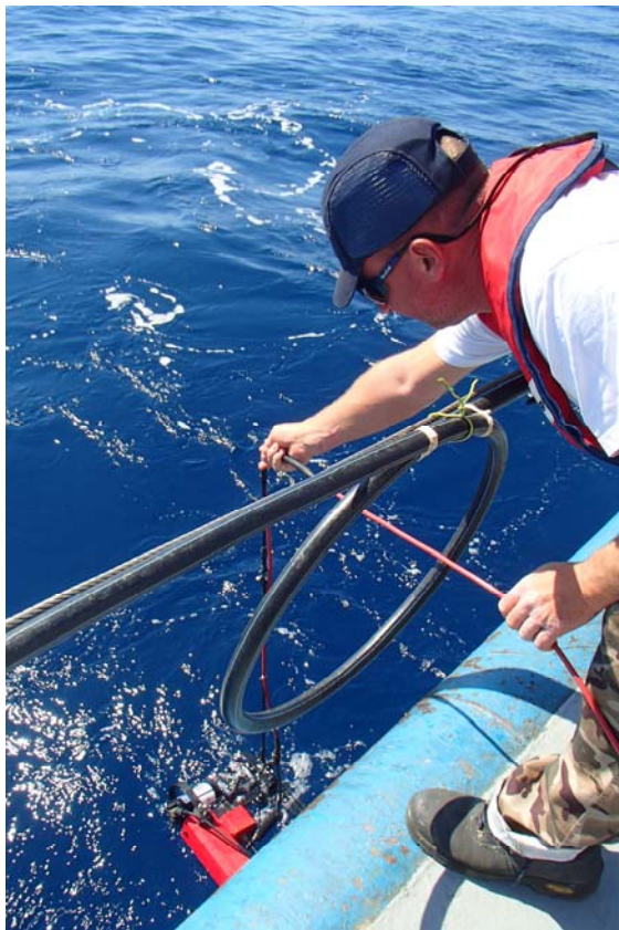
Deployment of the Compact Optical Profiling System (C-OPS) at the BOUSSOLE site.
