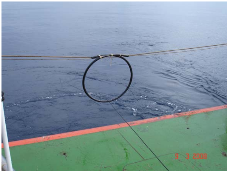
Fig 1. Plastic wheel replacing the pulley for deploying the SPMR.
