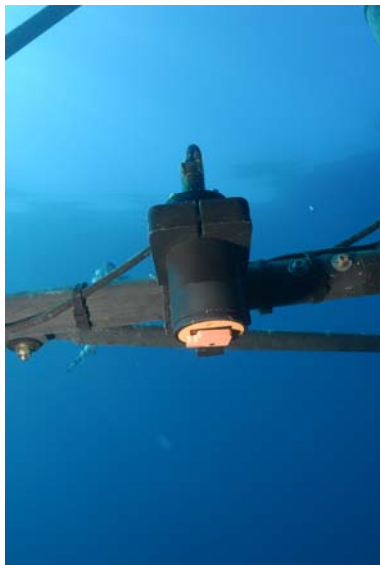
Fig 1. The WETLabs ® ECO FLNTUS fluorometer and turbidity meter, installed on the buoy since February 2007.
