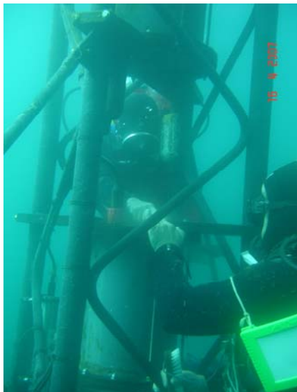
Fig 1. Divers Yves Lamblard and Christophe Lamoureux cleaning and checking the buoy instrumentation.
