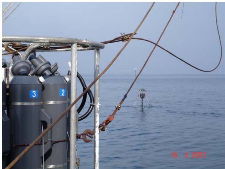
Fig 1. The BOUSSOLE cruise typical instrumentation: the buoy BOUSSOLE, the optical profiler SPMR hanging under the floating structure and the CTD rosette.
