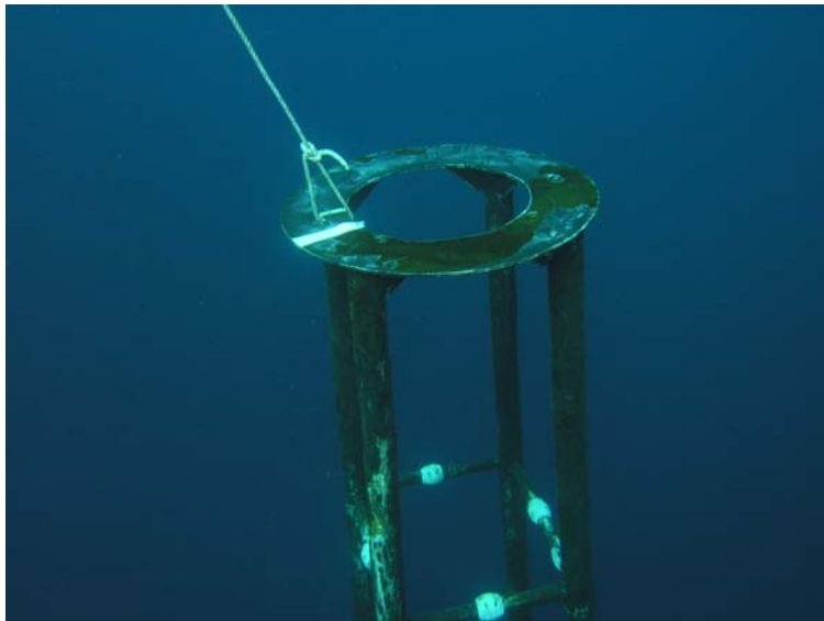
Fig 1. Only the lower structure of the buoy remains after the accident (collision with a boat ?) that occurred on February 12, 2007.
