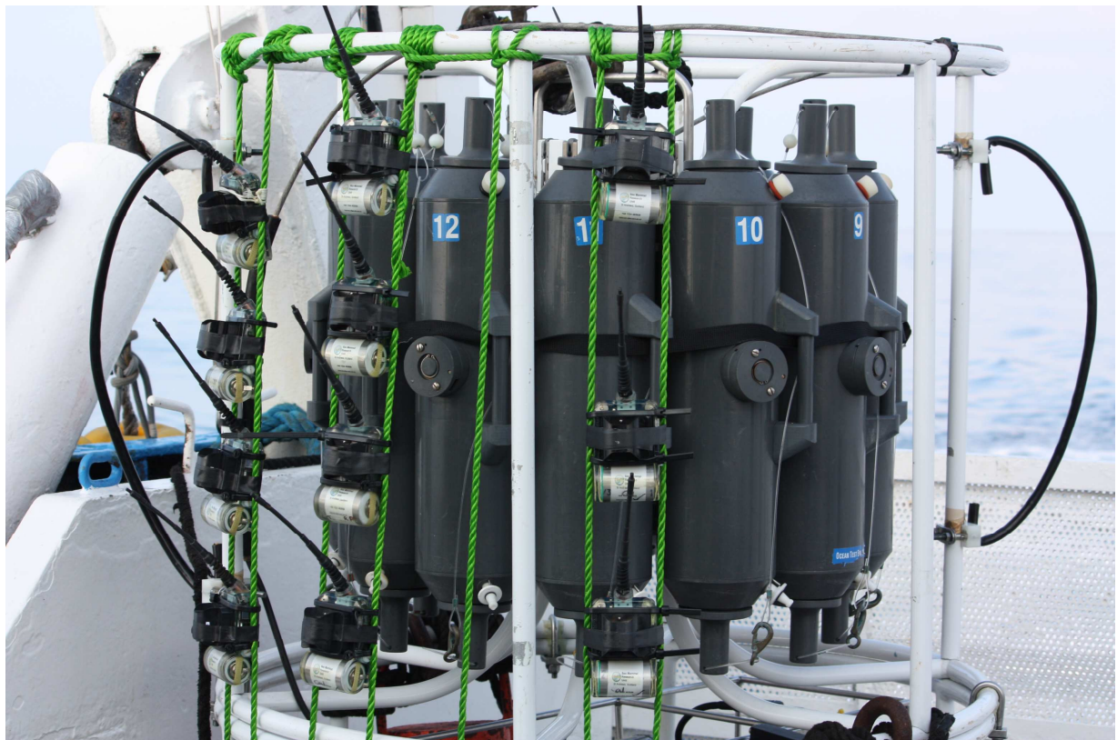
Autonomous CTD beacons to be later on deployed on Weddell seals in the Southern Ocean were affixed on the CTD Rosette for testing and for data intercomparison with the main CTD.
