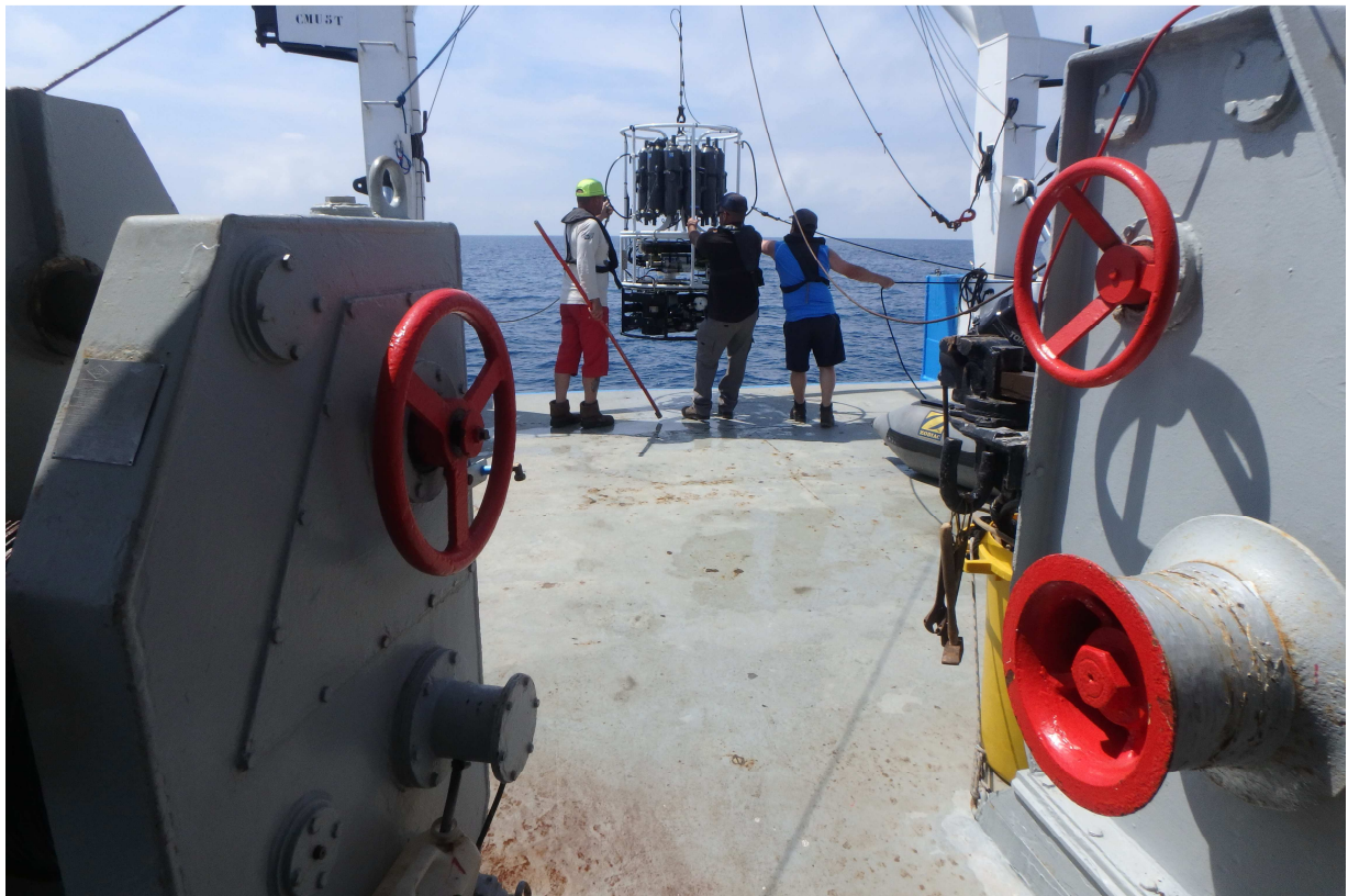
Deployment of the CTD Rosette at the BOUSSOLE site from the deck of the R/V Téthys II .
