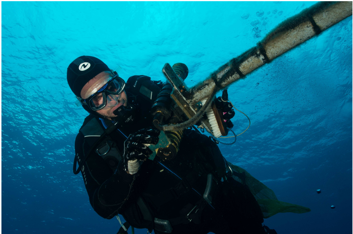
A diver is cleaning the hyperspectral sensors (measuring Ed and Lu ) on the BOUSSOLE buoy.
