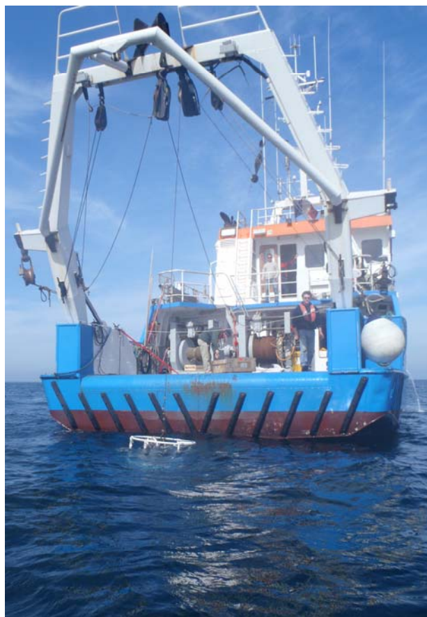
The start of a CTD cast with water sampling from the Tethys-II R/V stern
