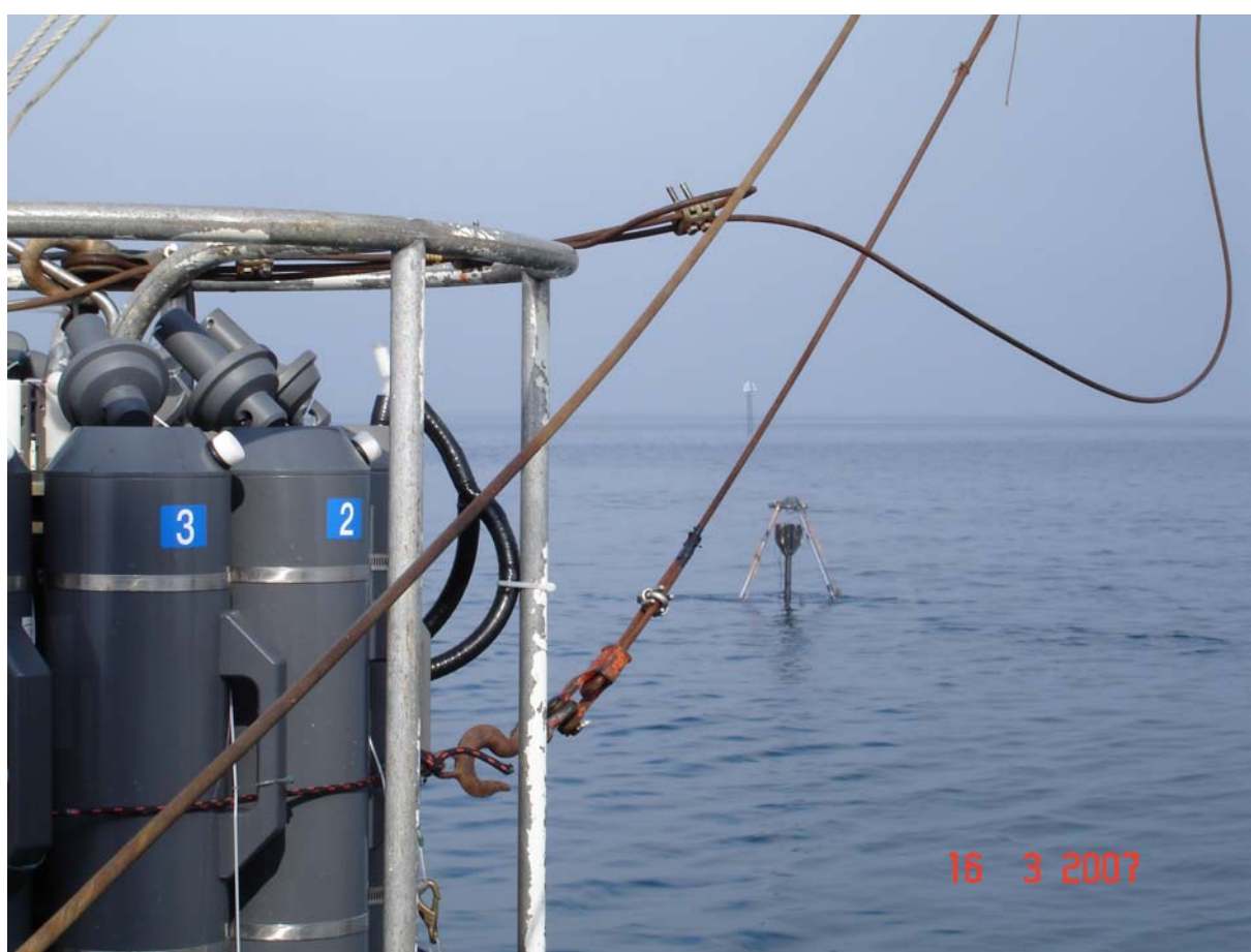
The BOUSSOLE cruise typical instrumentation: the buoy BOUSSOLE, the optical profiler SPMR hanging under the floating structure and the CTD rosette.
