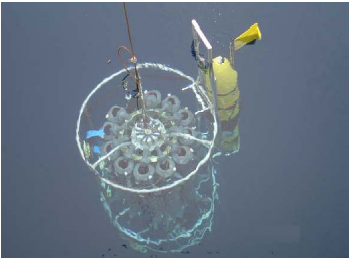
The SLOCUM glider fixed on the SeaBird carousel to inter calibrate the 2 CTD.
